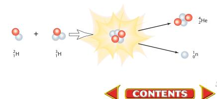
**FIGURE 31–7** The fusion of deuterium and tritium produces helium. Protons are red and neutrons are gray in the figure.
