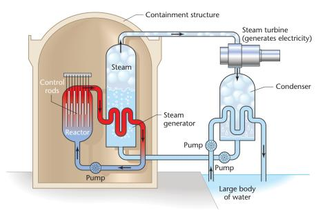
**FIGURE 31–6** In a nuclear power plant, the thermal energy released in nuclear reactions is converted to electric energy.
