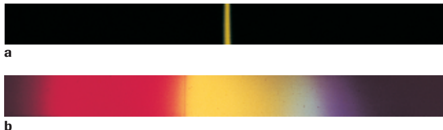
FIGURE 28-6 The emission spectrum (a) and the absorption spectrum (b) of sodium are pictured.
