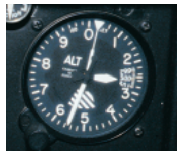
FIGURE 13–3 A tire gauge measures tire air pressure ( a ), and an aircraft altimeter uses pressure to indicate altitude ( b ).
